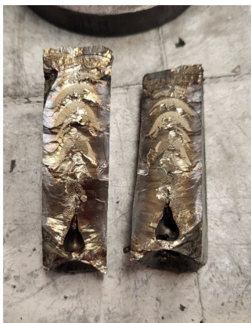
Fig. 5. Cracked LaNi5 alloy sample
