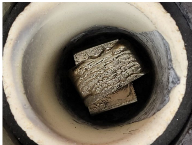
Fig. 4. Zirconia crucible with a metallic charge
