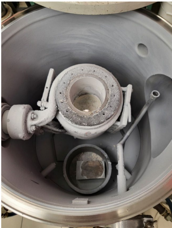
Fig. 1. Internal chamber of the Leybold Heraeus electric induction vacuum furnace
